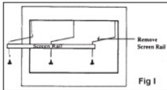
3. Remove the door from the box, and place into the opening of the firebox (finished side facing you), and align in position where it is to be installed. Make sure once set in place, it is level and plumb. We recommend you use a level to do this.
