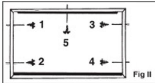
6. Remove the door from the opening, and using a 3/32" drill bit, drill the firebox where you had just marked for holes #1 through # 5.
